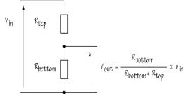
Figure 5: Voltage Divider Circuit
