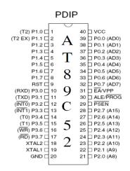
Figure 2: Pin Diagram of AT89C52
